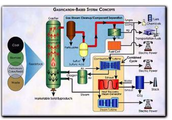
plasma arc gasification. Whether generated from conventional gasification or from plasma gasification, the syngas can be used in reciprocating engines or turbines to generate electricity or further processed to produce substitute natural gas, chemicals, fertilizers or transportation fuels, such as ethanol. Read more about the products of gasification.
