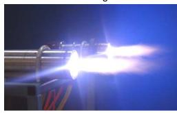
gas. The resultant flash from lightning is an example of plasma found in nature. Plasma torches and arcs convert electrical energy into intense thermal (heat) energy. Plasma torches and arcs can generate temperatures up to 10,000 degrees Fahrenheit. When used in a gasification plant, plasma torches and arcs generate this intense heat, which initiates and supplements the gasification reactions, and can even increase the rate of those reactions,
